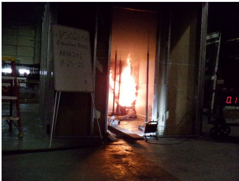
Photo No. 6 Horizontal Flame Propagation to 2 feet on Back Wall
